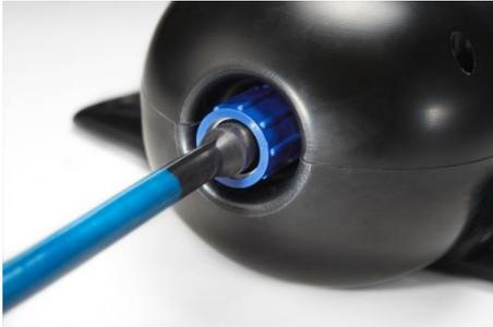
Connect the Connection Box to TrawlCamera, the 13pin connector can only be mated in the correct angle. Fasten the locking sleeve.
