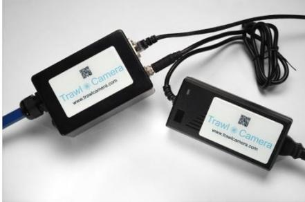
Connect the Power Supply to the Connection Box and tighten the nut on the connector. The light turns red, while the TrawlCamera is charging. The TrawlCamera is fully charged when the light turns green again. An empty battery will fully recharge in 5 hours.
